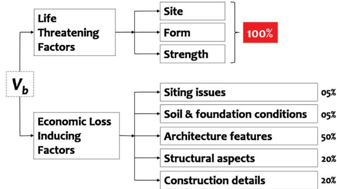
Figure 2.4: Flowchart for Vulnerability Estimation of a Building (values of Economic Loss Inducing Factors are given alongside the flowchart [ (Murty, Raghukanth, et al. 2012)]
