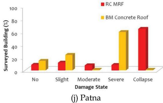
Figure 5.2: Possible Damage States of building typologies in the cities in seismic Zone IV cities with highest EDRI
