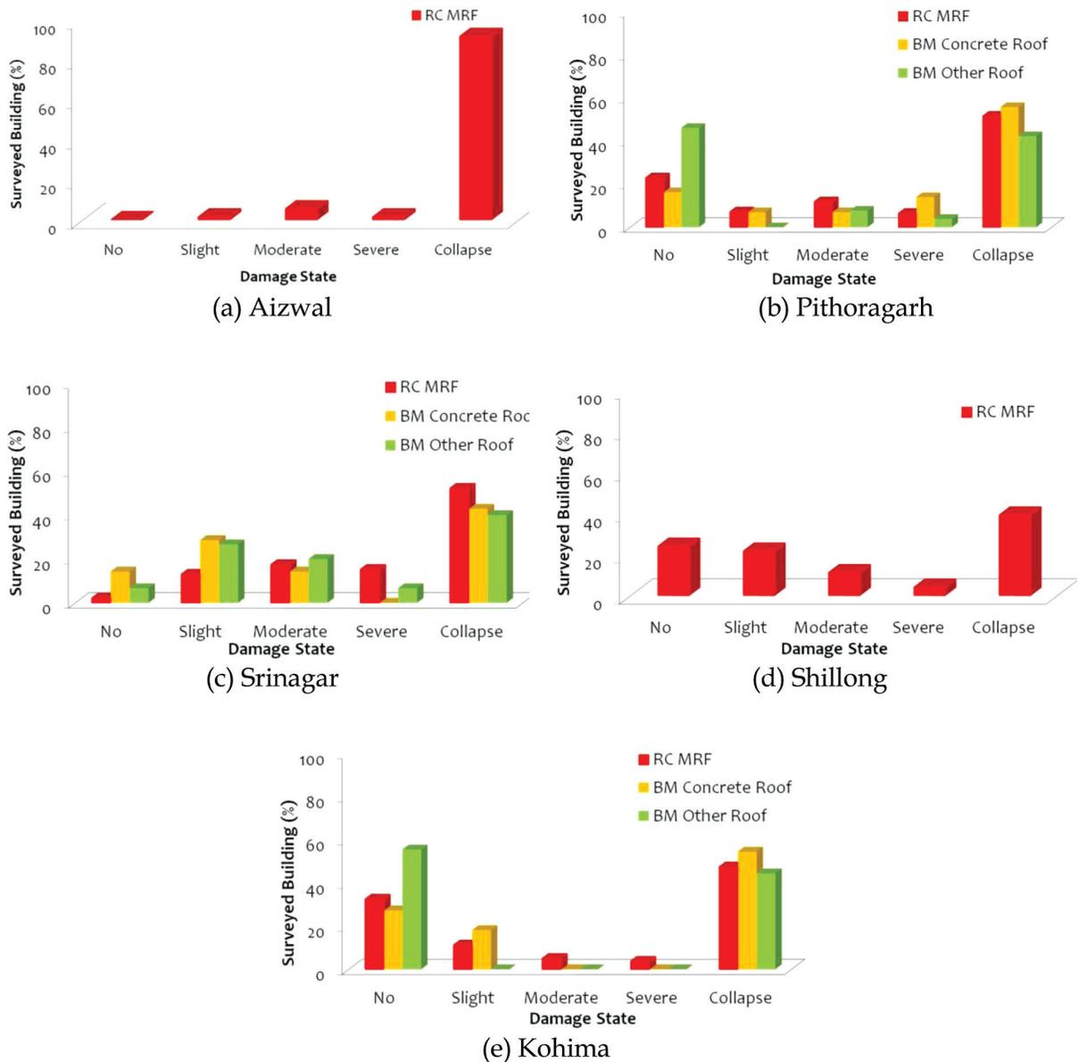
Figure 5.1: Possible Damage States of different building typologies in the cities in seismic Zone V with highest EDRI
