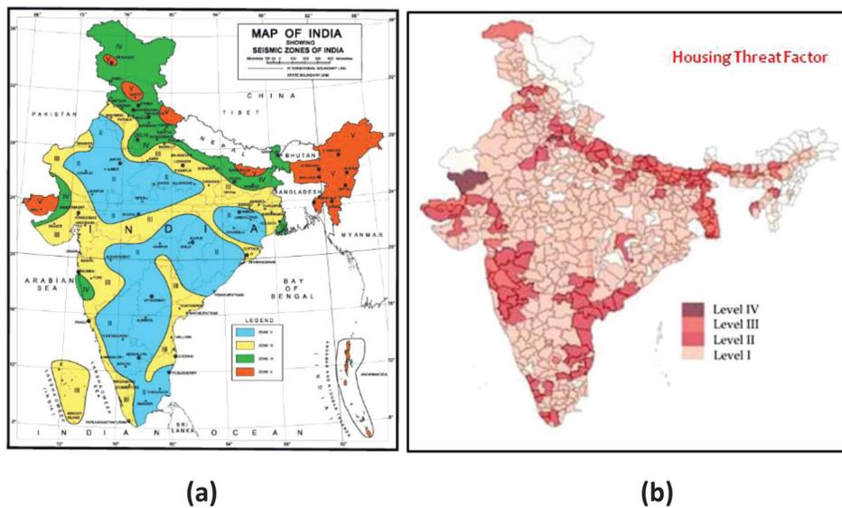
Figure 2.1: (a) Seismic Hazard Map [ (IS 1893(Part 1) 2016)], and (b) Housing Threat Factor [ (Ramancharla and Murty 2014)]
