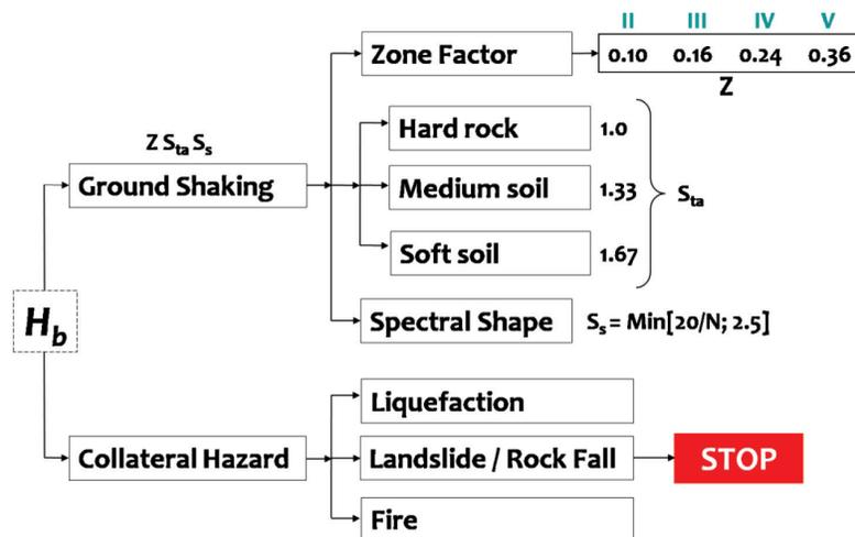
Figure 2.2: Flowchart for Hazard Estimation of a Building
