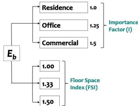
Figure 2.3: Flowchart for Exposure Estimation of a Building (values of Importance Factor  $I$  recommended in IS1893 (1) are given in brackets)
